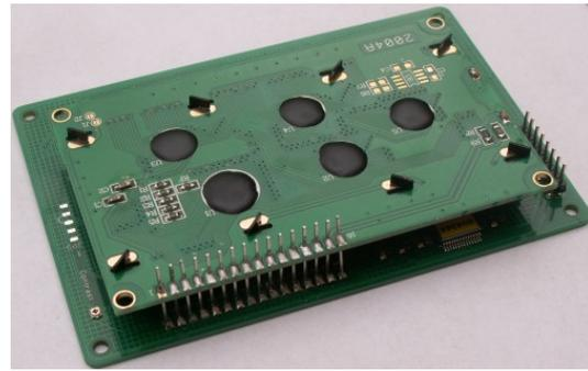
This will give a reasonable mechanical fixing but it is advisable to glue down the bottom of the display to the back of the PCB with hot melt glue.
